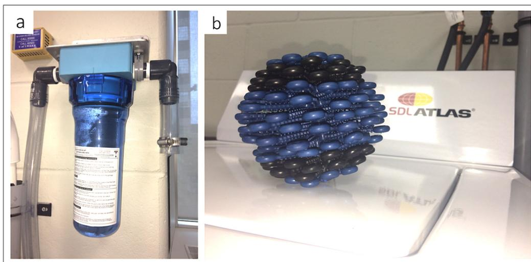
**Fig. 1.** (a) Lint LUV-R from Environmental Enhancements. (b) Cora Ball donated by Rachel Z. Miller of the Rozalia Project, on the SDL Atlas washing machine.
