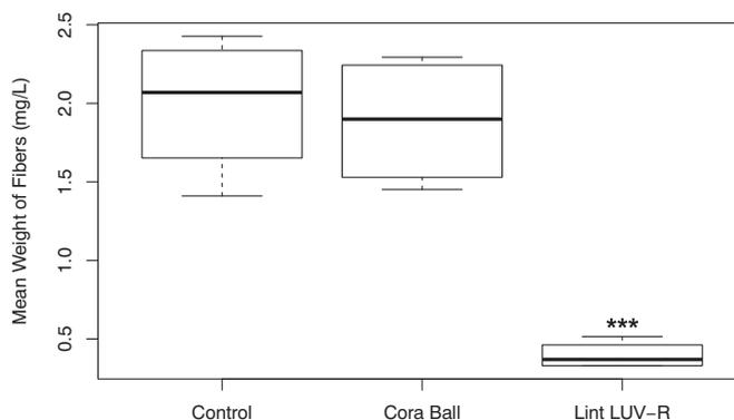
**Fig. 3.** Mean weight of microfibers in mg/L of washing machine effluent. One-factor ANOVA showed a significant difference across all treatments (p < 0.05). A post-hoc test showed significant differences between the Lint LUV-R and the control (\*p < 0.05; \*\*p < 0.01; \*\*\*p < 0.001; \*\*\*\*p < 0.0001). Boxes represent the first and third quartile, the line represents the median and whiskers represent the data range.
