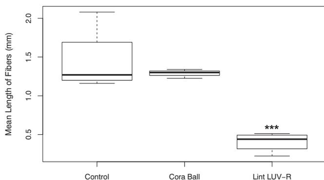
**Fig. 4.** Mean length of microfibers in mm in subsamples of effluent. One-factor ANOVAs showed a significant difference across all treatments ( $p < 0.05$ ). A post-hoc test showed significant differences between the Lint LUV-R and the control (\* $p < 0.05$ ; \*\* $p < 0.01$ ; \*\*\* $p < 0.001$ ; \*\*\*\* $p < 0.0001$ ). Boxes represent the first and third quartile, the line represents the median and whiskers represent the data range.
