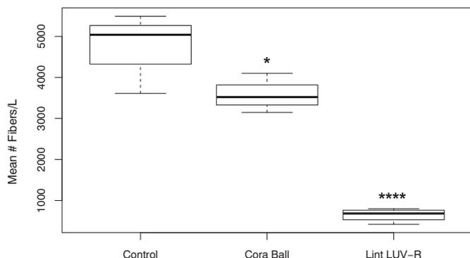
**Fig. 2.** Mean number of microfibers per L of washing machine effluent. One-factor ANOVAs showed a significant difference across all treatments (p < 0.05). A post-hoc test showed significant differences between both the Cora Ball and the Lint LUV-R compared to the control (\*p < 0.05; \*\*p < 0.01; \*\*\*p < 0.001; \*\*\*\*p < 0.0001). Boxes represent the first and third quartile, the line represents the median and whiskers represent the data range.
