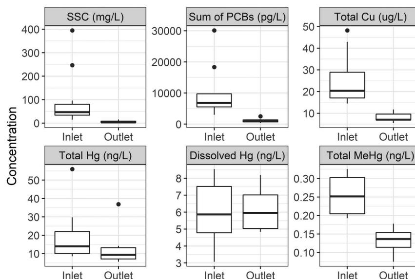
**Fig. 2.** Box and whisker plots showing the resulting data from water quality samples collected in storms during water years 2012, 2014, 2015, and 2017. The range, mean, quartiles, and data outliers for the six analytes are shown for both the inlet and outlet. One inlet PCB sample is not represented on the graph; it is 226,000 pg/L.
