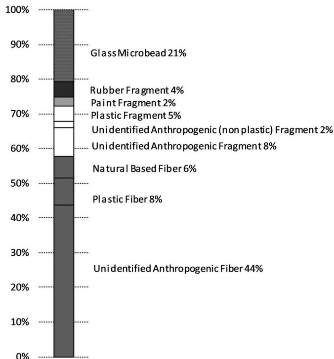
**Fig. 3.** Microparticle composition of inlet samples ( $n = 3$  storms).
