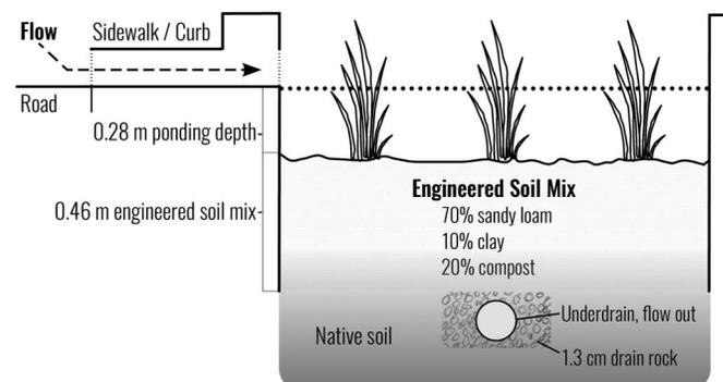
Fig. 1. Cross-section of the bioretention rain garden.
